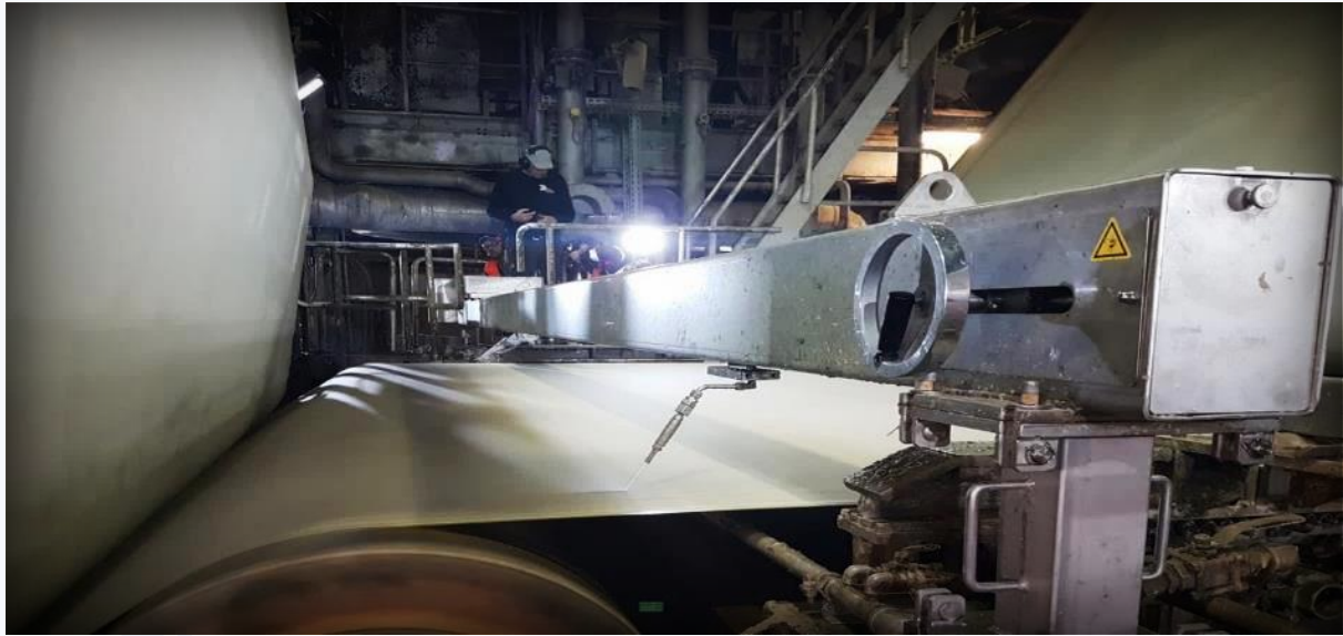
PCF Tail Cutter for wet section in operation
