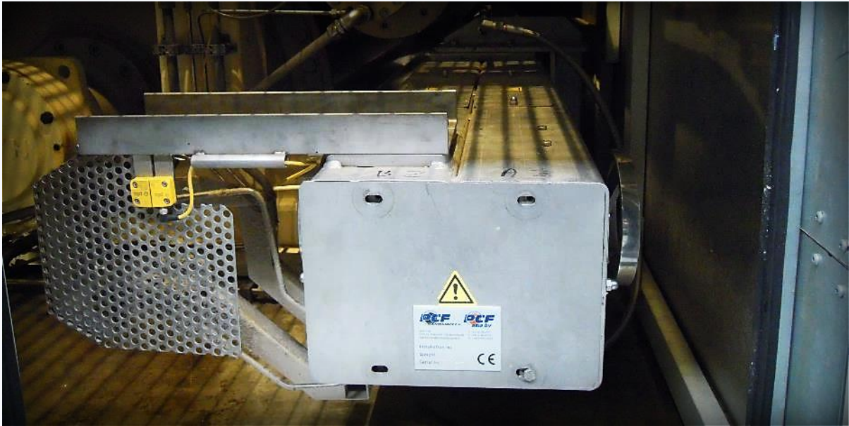
PCF Tail & Deckle Cutter for dry section, with HP water needle jets in operation
