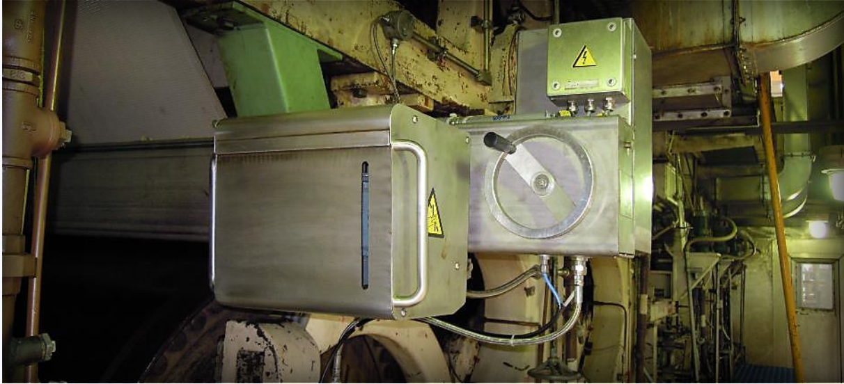
Tail Cutter for dryer section with Rotating Knife in operation
