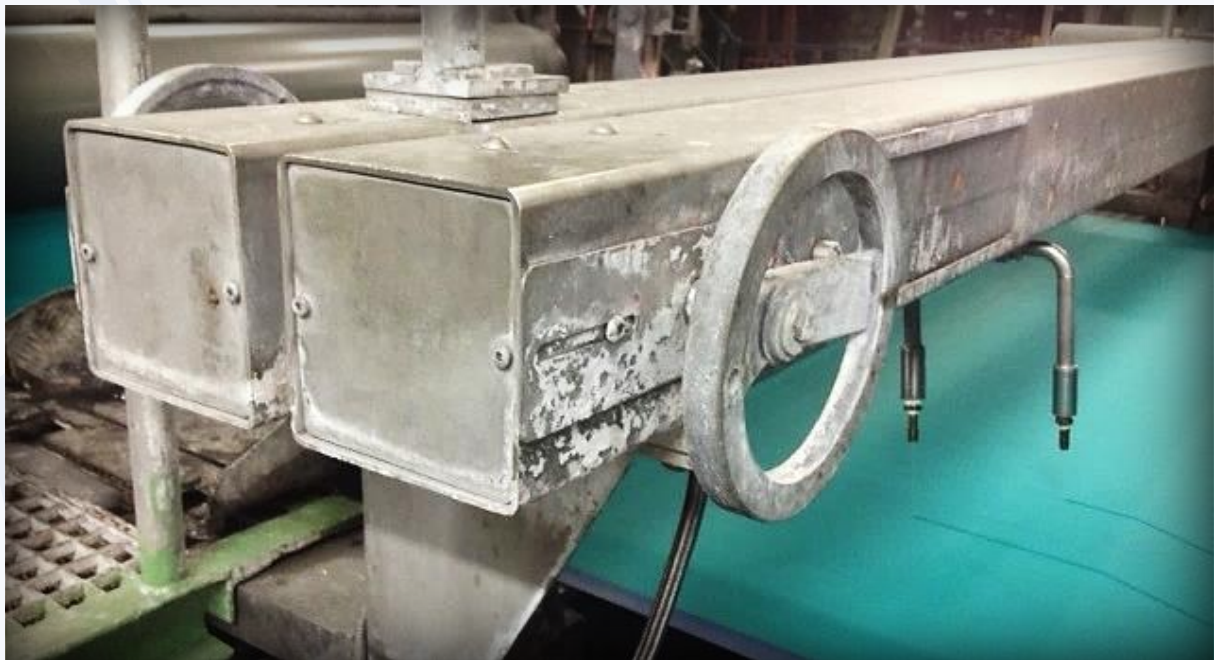
PCF Tail & Deckle Cutter for wet section in operation
