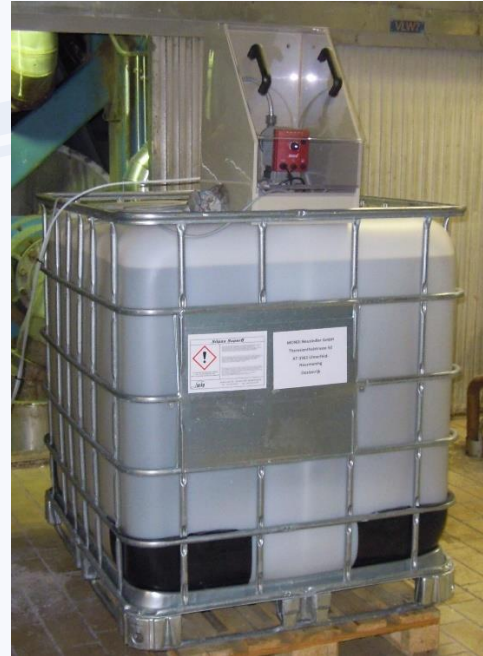
PCF PF69 silicone fluid tank with dosing pump
