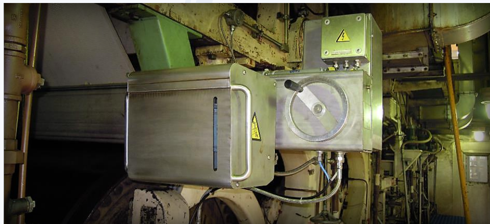
PCF Tail Cutter for dryer section with Rotating Knife in operation
