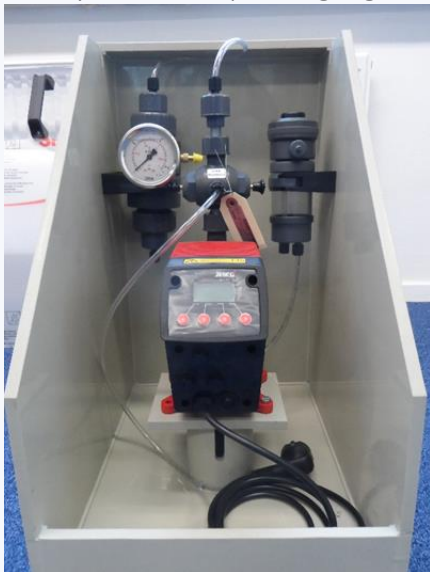
Dosing pump unit
