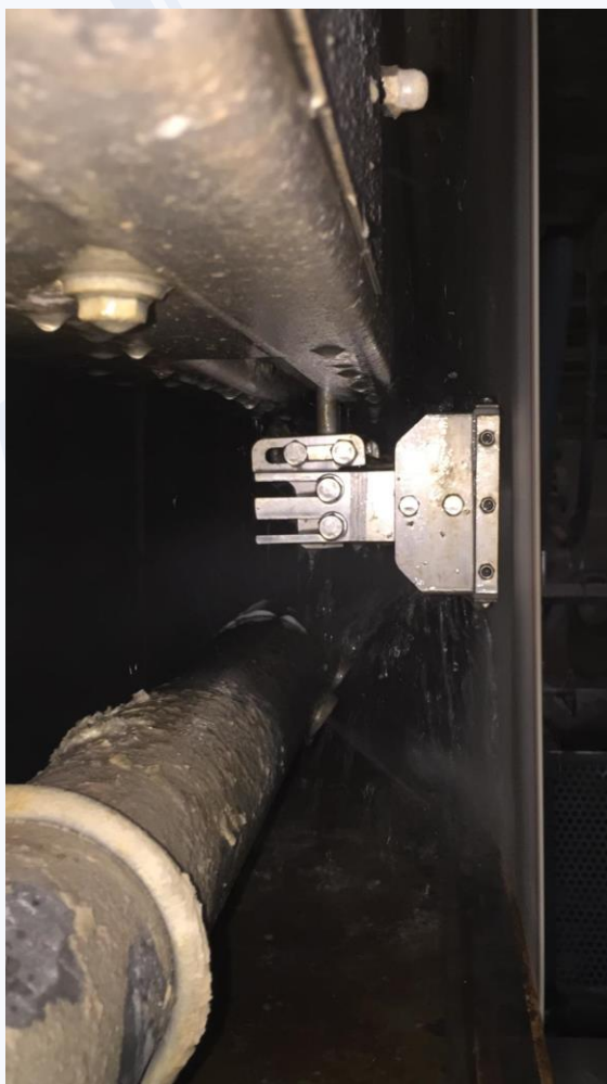
Cleaning with oscillating showers results in stripes on the press felt
