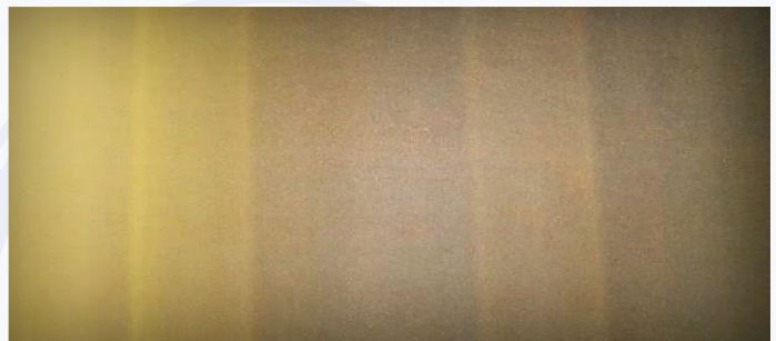
Cleaning with oscillating showers results in stripes on the press felt
